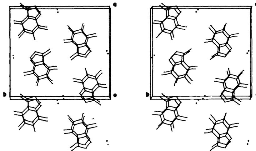
**Figure 2.** Stereopair drawing of the crystal packing of caffeine monohydrate viewed perpendicular to the (001) face.<sup>14</sup> The oxygen atoms of the water molecules are designated by dots.
